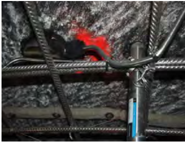
Total pressure sensor and pore pressure sensor on rock surface
