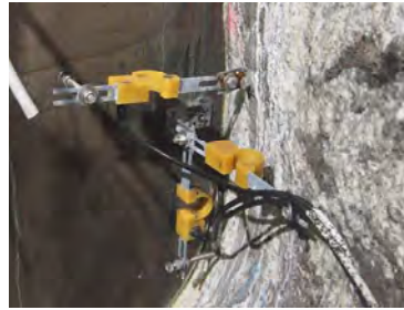
Displacement sensors at the front face of the plug
