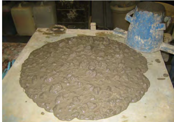
DIN flow of Binary (FIN) mix design, SCC.
