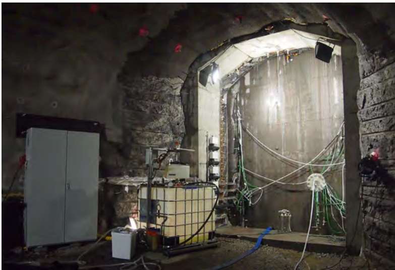
Leakage measurement system at front face of plug during pressurization test
